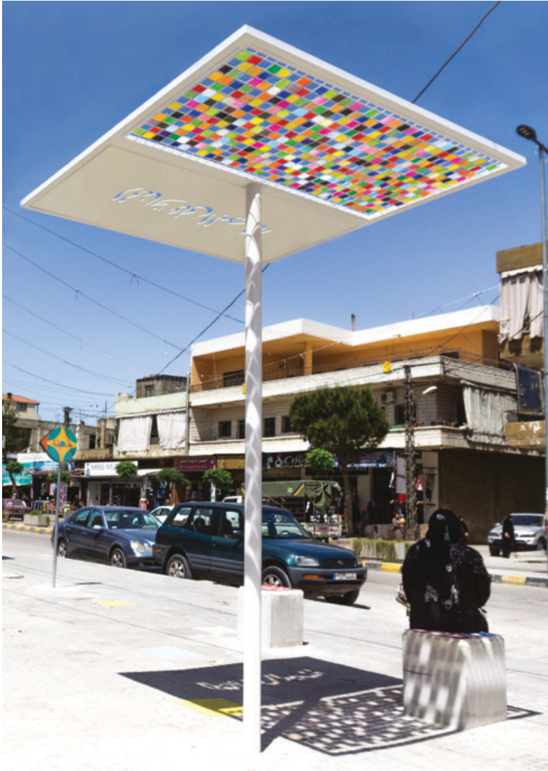
Figure 5.5 Shade incorporating laser-cut phrases and recycled materials above newly installed seating. A sign in the background points passers-by to the revitalised garden.
